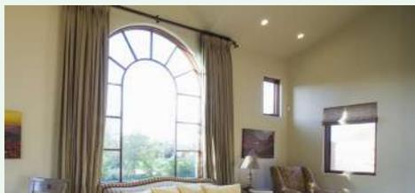
Bespoke secondary glazing can also be provided for windows of an unusual shape, such as traditional properties. The timber subframe and aluminium frame can be shaped from straight to curved lines to match the original window. This is a great option for listed and older buildings as it allows the original window characteristics to remain in place.
